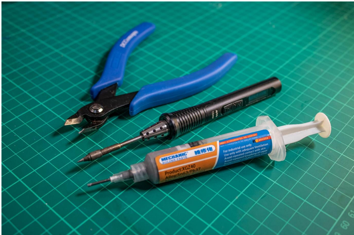
Recommended Tools: Flush cutters, Soldering Iron, Solder / Solder Paste.
